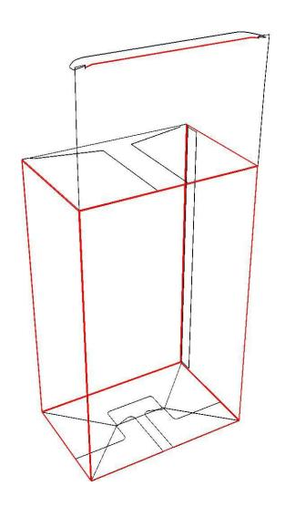
**Glue Panel** Top Panel Side Panel Side Panel **Back Panel** Front Panel "U" Flap Side Flap **Tongue Flap** Side Flap
